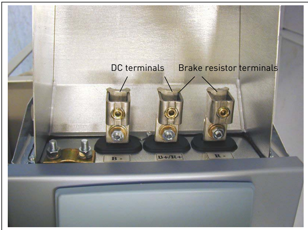
Figure 6-19. Brake resistor terminal box on top of FR8
