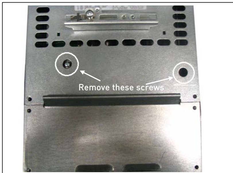
Figure 6-3. Changing of EMC protection class, FR6. The cable cover does not need to be removed
