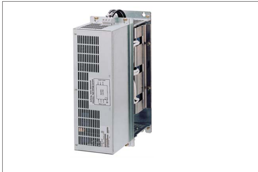
Fig. 7-15 Construction with an adapter set
